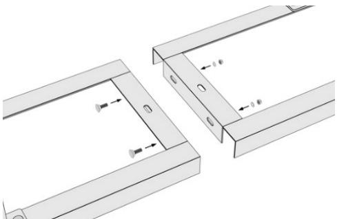
**7** • Lock the frames using bolt, washer and nut.
