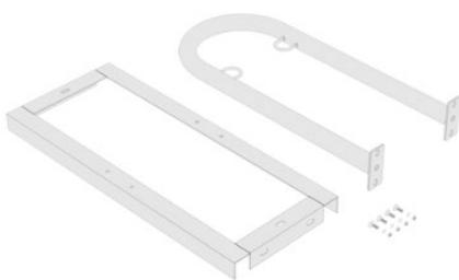
**2** • Place the hoop on the frame with mounting points facing upward.
