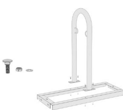
**3** • Attach the hoop to the frame using a bolt, washer and nut.
